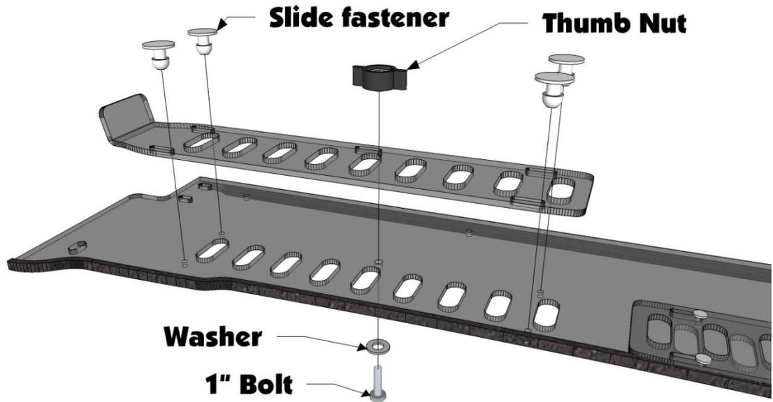
4. Now clamp the bottom section to the Teryx. The windshield should be clamped as shown in the image below.
