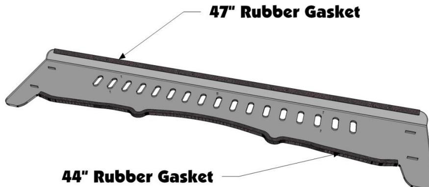
3. Next install the sliding vent panel to the bottom section as shown in the image below.
