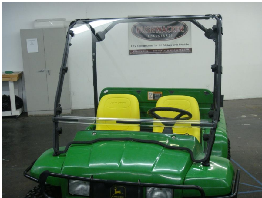
Figure 7.1 - Remove windshield plastic protective paper
