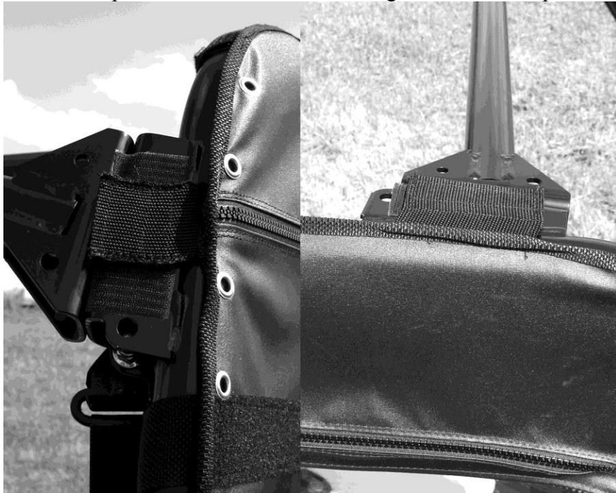
6. The bottom of the door has magnets sewn to the edge that will hold to the metal floor pan. Towards the rear of the door are three magnets that will wrap underneath the floor pan and attach the inside as shown in the photo below.
