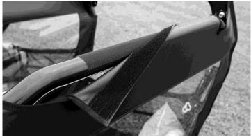
11. The sides of the rear window will attach to the double-sided Velcro tabs that hold the rear of the doors in place.
