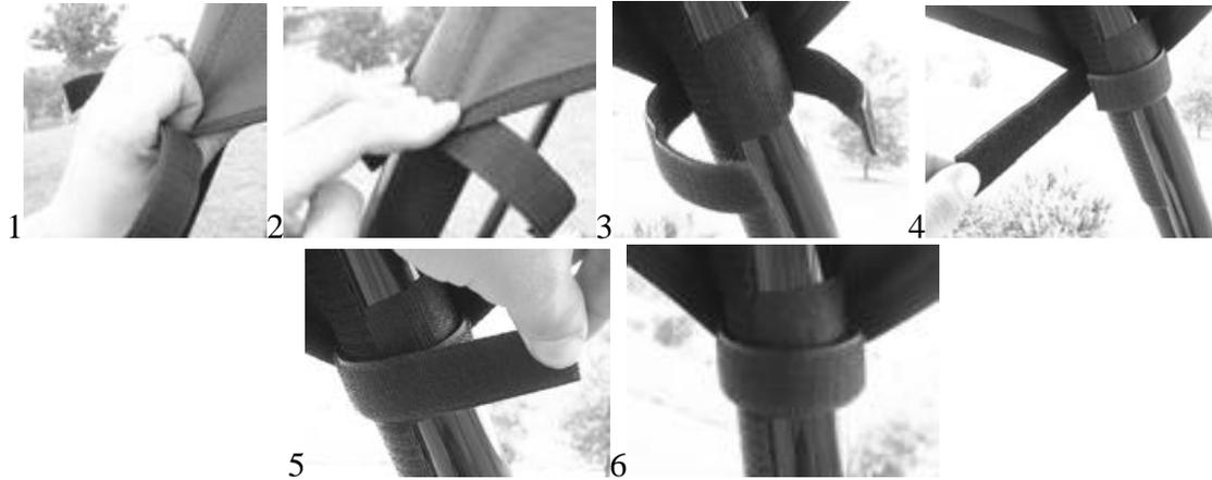
6. Now note the positions of the three Velcro tabs on both sides of the windshield and attach the correct size adhesive Velcro strips the roll cage as shown in the photo below. After attaching the strips pull the windshield tight side to side by attaching the Velcro tabs to the adhesive strips creating a tight wrinkle free surface to the windshield.
