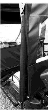
7. Now start at the bottom and attach the rear window making sure that it is centered. Then pull it up and attach the top and the sides last.
