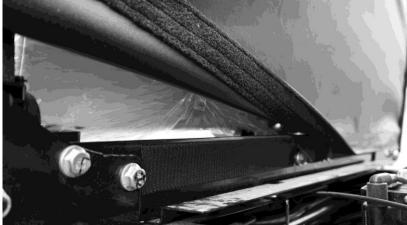
5. Next attach a piece of adhesive Velcro across the top bar, it should be placed on the top slightly angled towards the front of the vehicle. See Photo below.
