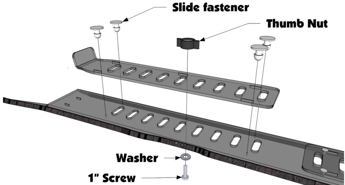
6. Now you are ready to place the windshield on the vehicle. With assistance, place the upper windshield on the frame. Wrap the clamps provided around the steel frame tubing at all slot locations. Now place the bolts and washers through the slots with washers on the inside of the windshield on top of the clamps. Run the bolts through the clamps on the backside, and install a thumbnut on the outside of the windshield to secure. Repeat with the lower windshield. See Diagram Below.
