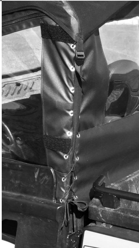
13. Now take the Top Cap and place it over top of the vehicle and the enclosure. Make sure that it is centered and then take the straps and run them through the ladder lock buckles sewn in the corners and pull them tight. The straps lace through the buckle as shown in the diagram below.
