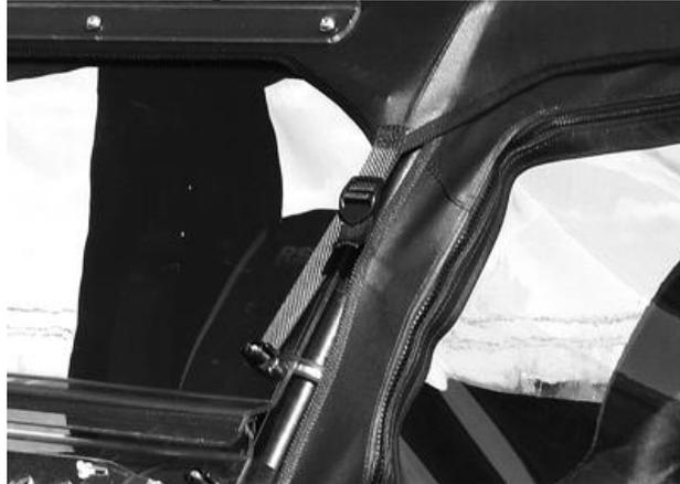
12. Now take the two straps sewn to the Velcro and attach them on the rear bar under the cab enclosure. This part can be a bit complicated but is not impossible. Find a good spot between the lacing and wrap the double-sided Velcro around the bar after placing one of the 3" adhesive Velcro strips on the backside. Then run the webbing through the lacing and up towards the top cap. When finished, it should look like the photo below.
