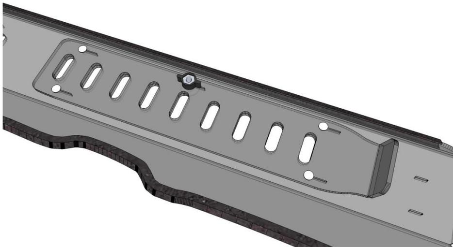
5. Now install the lower portion to the upper portion using the nylon bolts. There are Nine holes in both section with the holes in the upper portion being bigger. Set the upper portion on top of the lower portion and screw them together making sure that the slots on the ends are lined up. The photo below shows how this looks.
