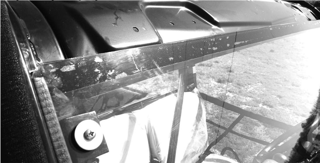
8. It's time to install the windshield on the vehicle. There are two slots on either side, they get attached to the vehicle using the bent metal brackets provided. To do so start from outside in with a 1 1/4" bolt, large metal washer and large rubber washer. Put these in the slots from the outside. Then place the metal bracket on the inside so that it wraps around the frame and the bolt is in hole. Lastly put a small washer and lock nut on the bolt and tight. See photos below
