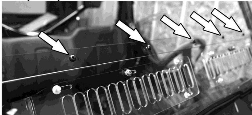
6. Now install the 11" and 19" side bulb gaskets on the sides of the windshield above and below where the windshield was screwed together and where it is double thickness.
