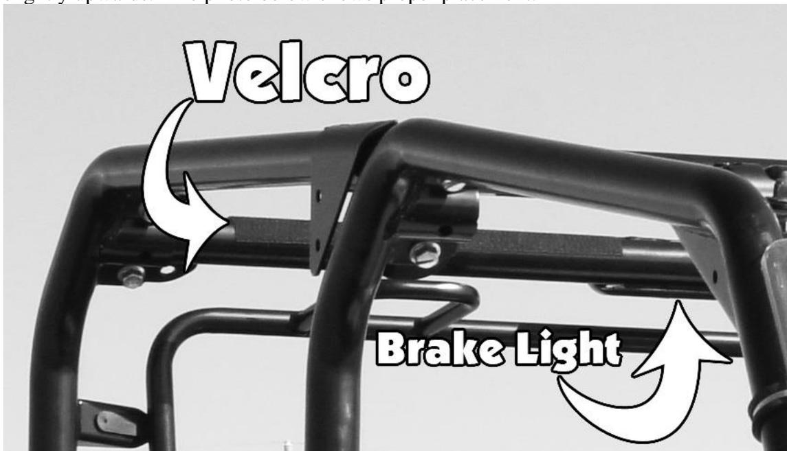
5. After placing the Velcro on the roll cage, attach the rear window. Across the top of the rear window is a cutout for the brake light, line this cutout up with the brake light and attach the rear window to the adhesive Velcro. See Photos Below:
