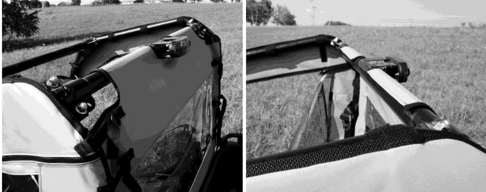
6. Next step is to attach the sides of the rear window to the roll cage. There are 5 strips of double-sided Velcro sewn perpendicular to the edge of the panel. Take the 6" adhesive Velcro strips and wrap them around the bars where each double-Sided Velcro strip lines up. Then wrap the double-sided Velcro around the adhesive strip on the bar. The photos below show how this works.
