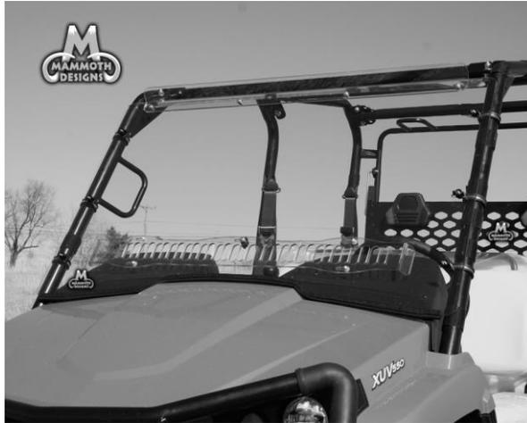
10. Once the Lexan Windshield is in place it's now time to install the roof panel. Included in your package are two sets of webbing straps. One set has grommet holes in one end and these are used for the front of the top. The other set has double-sided Velcro sewn to one end and is used for the rear of the top.
