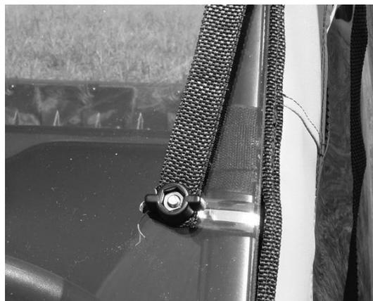
12. Now take the strap and run it through the buckle sewn to the corner of the top. Do not pull tight until all straps have been attached. See Photos Below:
