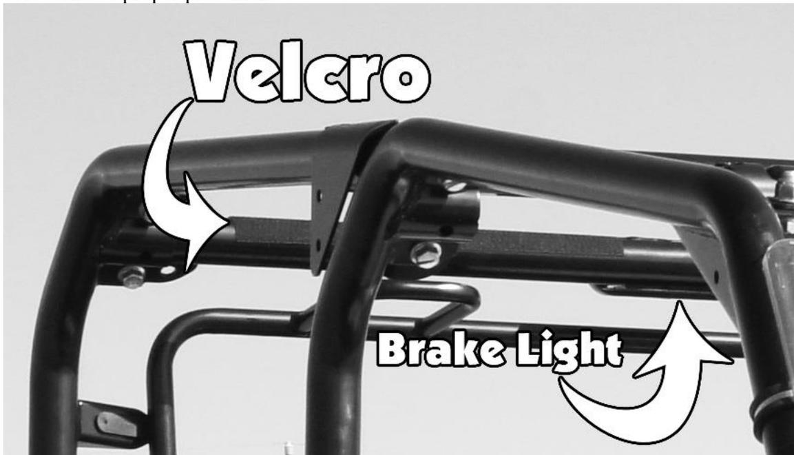
7. After placing the Velcro on the roll cage, attach the rear window. Across the top of the rear window is a cutout for the brake light, line this cutout up with the brake light and attach the rear window to the adhesive Velcro. See Photos Below:
