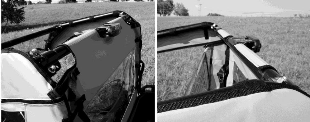
8. Next step is to attach the sides of the rear window to the rear doors. Sewn to the rear window are straps with buckles and sewn to the rear doors are loops. Take the strap on the rear window and run it through the loop on the rear doors. Then take the strap back through the buckle and pull tight. Do not over tighten to the point that the rear window is pulled more to one side than the other; you may have to adjust them until the rear window is centered correctly. See photo below:
