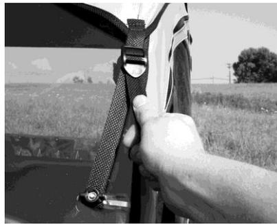
13. Once the front straps have been attached to the windshield move to the rear of the vehicle and attach the webbing straps with double-sided Velcro to the rear bar between the rear door and the rear window. First wrap the bar with the adhesive Velcro and then wrap with the double-sided as you did with the front and rear doors. Two extra straps have been provided for top only usage. See photo below:
