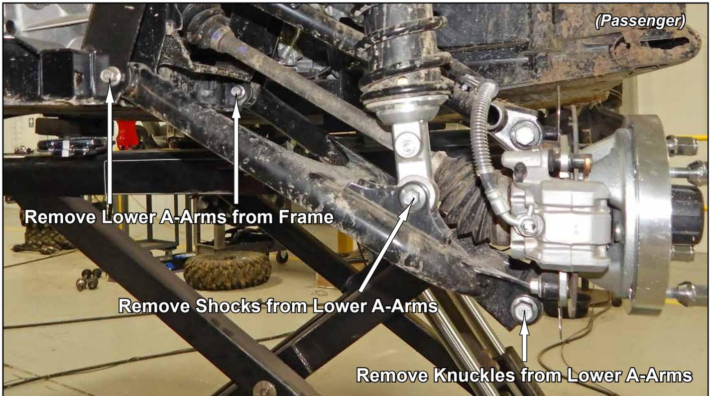
SuperATV recommends using thread locker on nuts when securing components.
