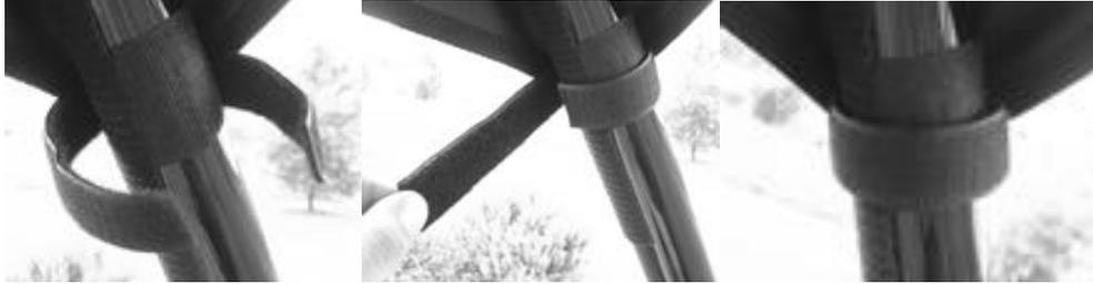
5. Now move to the rear of the cab and you will see that a strip of Velcro is sewn across the back and should be lined up with the bar running behind the seats. Clean the bar and take the 45" adhesive Velcro strip and apply it to this bar trying to center it as much as possible. Attach the Velcro sewn into the enclosure to it.
