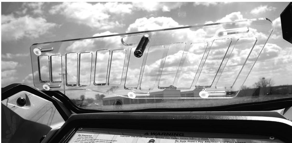
6. You are now ready to install the windshield on your roll cage. Place the windshield on the vehicle first. Begin with the Bolts in the top corners of the windshield. Using a 1" bolt two washers and a lock nut fasten them as shown in the photo below.
