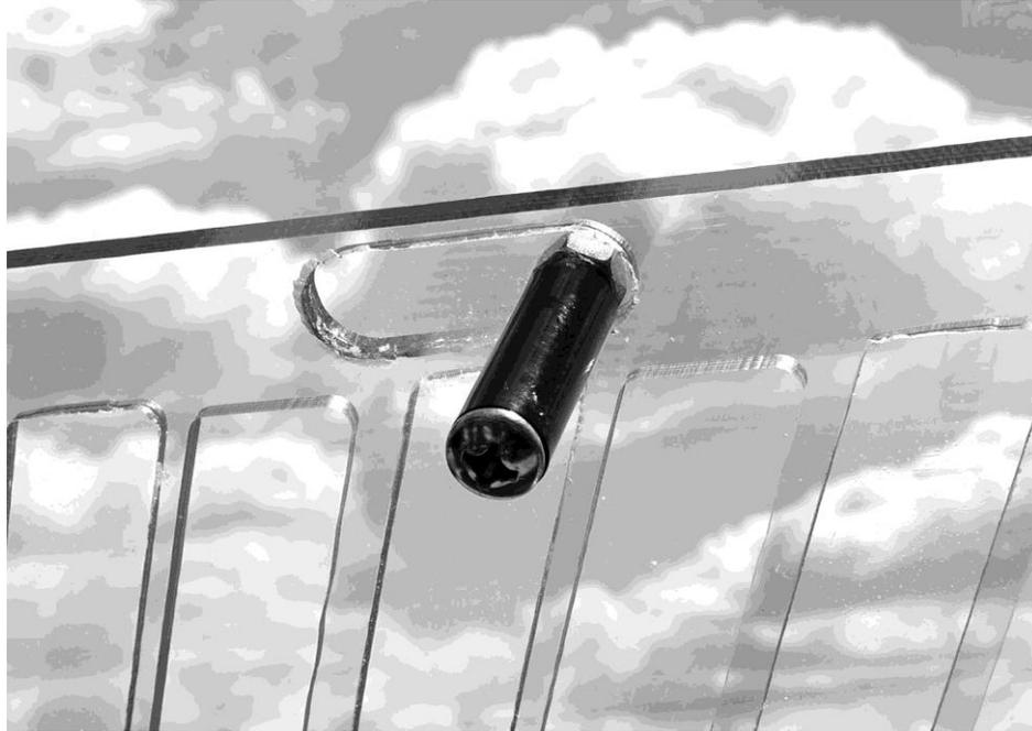
Now insert the bolt in the small holes and screw on the lock nuts so the end of the bolt is flush with the outside edge of the lock nut. **Make sure that you place the bolt through hole on each slider so that they are mirror images of each other.**
