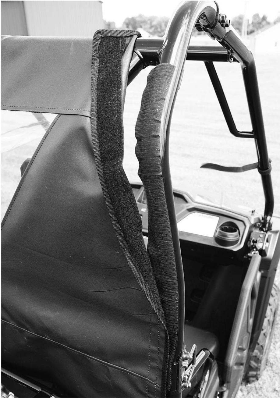
**12.** Now just hang the rear window from the Velcro on the top bar and attach it down the sides. The bottom of the rear window has magnets that will attach to the frame.
