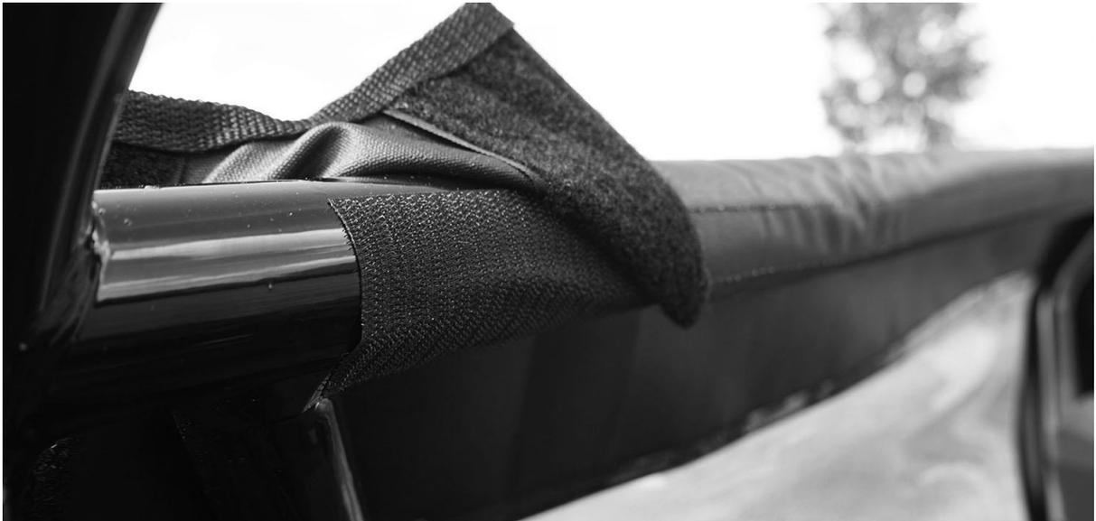
11. Next attach the sides to the double-sided velcro tabs sewn along the rear of the doors as shown in the photo on the next page.
