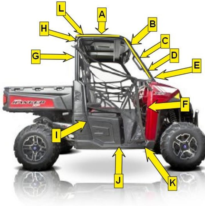
**Step 3:** After all adhesive hook strips are attached, begin attaching the enclosure to the cab frame. As you attach the hook and loop, square each panel to the frame. **PLEASE NOTE, FOR MAXIMUM ADHESION, ALLOW THE ADHESIVE HOOK TO ADHERE TO THE FRAME FOR 24 HOURS BEFORE PULLING AGAINST THE HOOK WITH THE LOOP STRIPS.**
