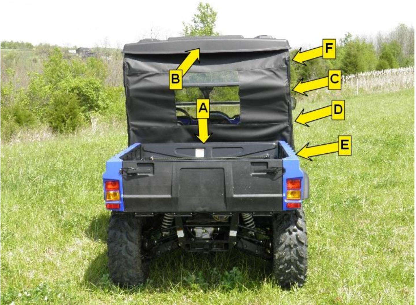
**Step 3:** After all adhesive hook strips are attached, begin attaching the enclosure to the cab frame. As you attach the hook and loop, square the enclosure to the frame. **PLEASE NOTE, FOR MAXIMUM ADHESION, ALLOW THE ADHESIVE HOOK TO ADHERE TO THE FRAME FOR 24 HOURS BEFORE PULLING AGAINST THE HOOK WITH THE LOOP STRIPS.**
