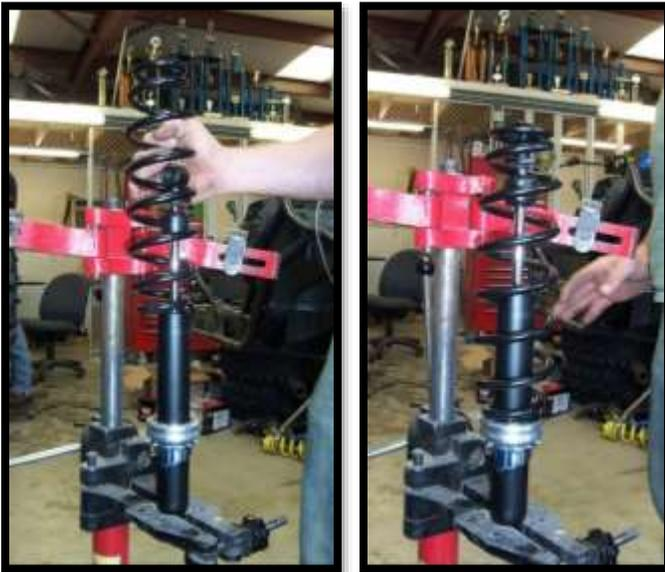
g) Compress the spring and place retaining clip back on the shock.
