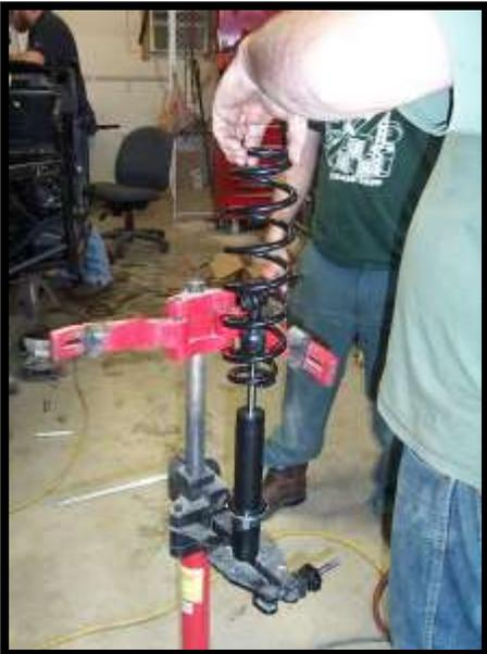
e) Slide the spring lift bracket (58Z) onto the shock.
