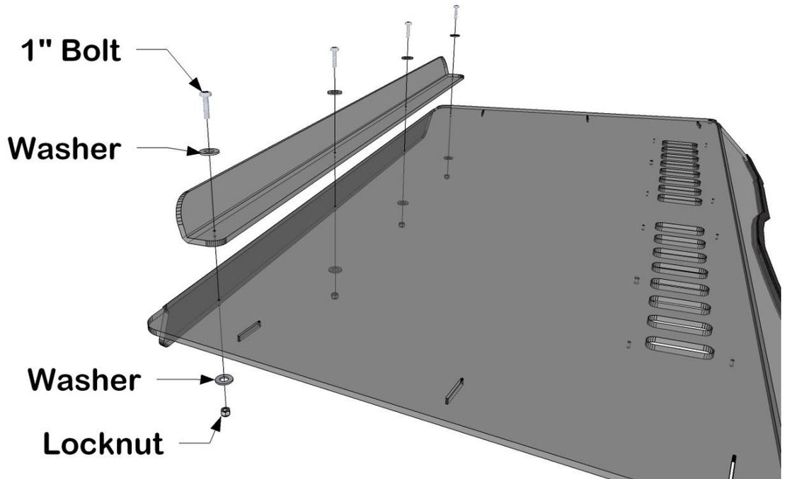
8. If you are using this windshield with a Over Armour Cab enclosure then you will use the Top Brace to sandwich the cab material and seal off the inside from the wind. The diagram below shows how it will work.
