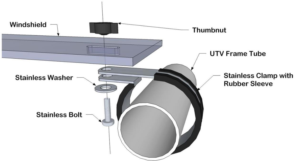
7. Now you can install the top brace if you want. If you do not have a Over Armour Cab enclosure to work with this windshield, the top brace is not needed but can be installed for extra strength. Below is a diagram showing how the brace is to be installed.
