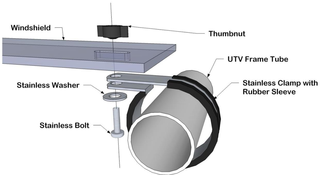
7. Now you can install the top brace if you want. If you do not have an Over Armour Offroad Cab enclosure to work with this windshield, the top brace is not needed but can be installed for extra strength. Below is a diagram showing how the brace is to be installed.
