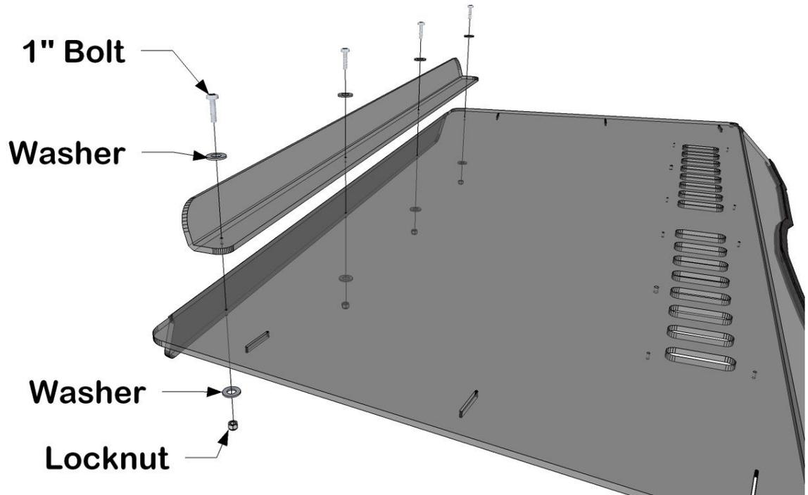
8. If you are using this windshield with an Over Armour Offroad Cab enclosure, then you will use the Top Brace to sandwich the cab material and seal off the inside from the wind. The diagram below shows how it will work.
