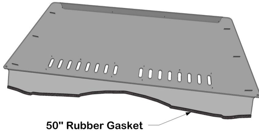
4. Next install the sliding vent panel on the inside of the windshield as shown in the diagram below. To install slide fasteners, push through holes with thumbs until it is completely through the hole in the windshield and locked in place.
