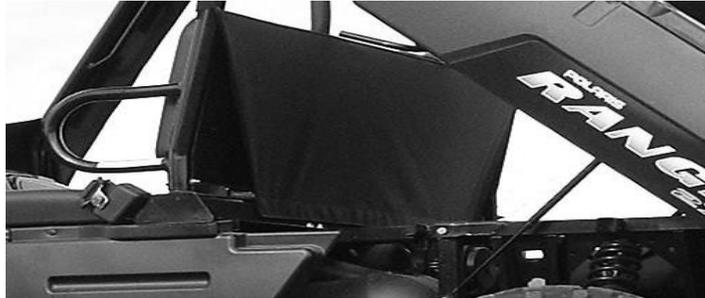
7. Next place the six 5” adhesive Velcro strips on both sides of the rear window to match up with the corresponding tabs.
