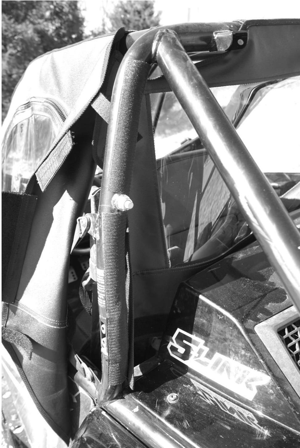
3. Next take the 8" adhesive Velcro strip and place it on the front fender as shown in the photo below. Then affix the bottom of the front panel to it as shown in the second photo.
