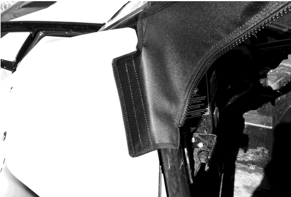
4. Last part of the door to attach is the bottom to the factory half-door. Take the 44" adhesive Velcro strip and attach it to the factory door to match up with the Velcro sewn to the bottom of the soft doors. The adhesive Velcro will cross the hinge of the door, take a knife and cut the adhesive Velcro at the hinge.
