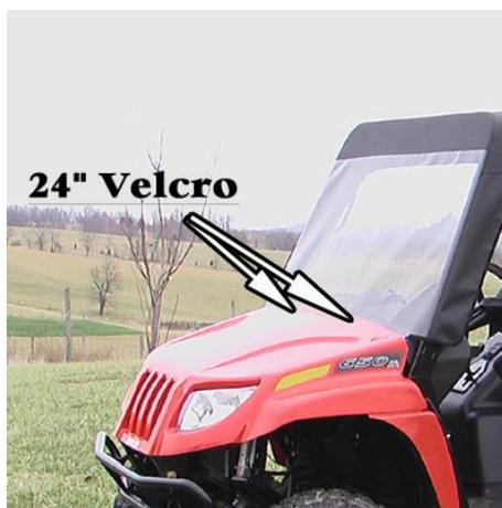
5. Working your way to the rear of the roll cage carefully fit the Cab into position. Pull down in the corner to approximate the position for the 12" Velcro strip and wrap it around the roll cage. Now pull down on the corner and wrap adhesive Velcro with the double-sided strip sewn to top.
