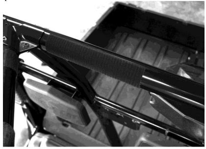
5. Now take the rear window and attach the two 8" tabs to the adhesive Velcro centering the cutout across the top under the rear brake light. The photo below shows how it should look.
