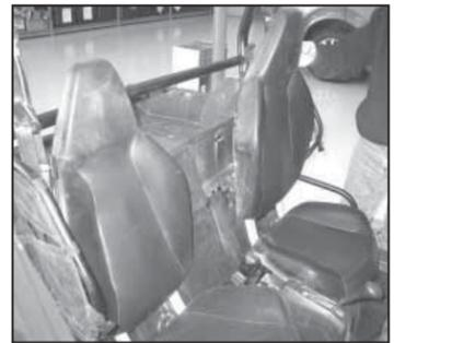
42. Re-install the driver and passenger seats as shown.
