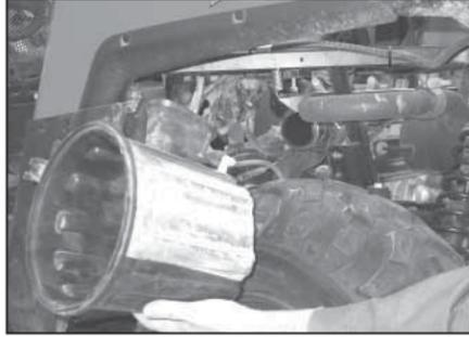
19. Remove the air box assembly as shown.
