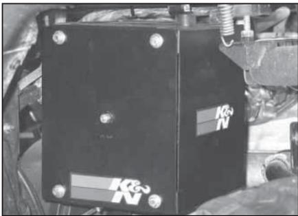
32. Install the K&N® air box cover, aligning the 1/4" bolt in the filter with the center hole in the cover on the K&N® air box. Secure with the provided hardware as shown.
