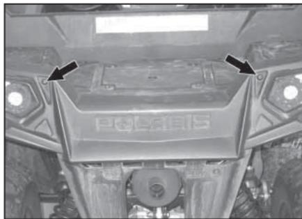
38. Re-install the two bolts securing the rear of the cargo bed as shown.
