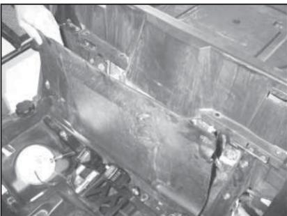
4. Pull firmly to remove the engine splash cover as shown.
