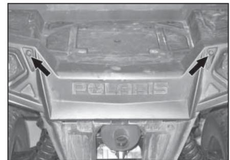
8. Remove the two torx bolts at the rear of the cargo bed as shown.
