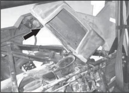
14. Remove the intake cover as shown.
