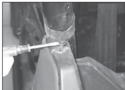
6. Remove the push pins behind the roller bar (one on the right and left side of the cargo bed) as shown.
