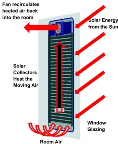
This SIS model air solar heater heats air. It is like an electric room convection air space heater except it is operated by the sun's solar energy. Hang or set it in a sun facing window, or side-ways, or even upside down, and it will maintain heat in a large room or area in the home. The heating capacity is equivalent to a 150 to 500 watt electric heater, depending on the daytime sun and cloud cover.
