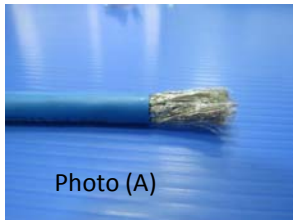
Strip off cable jacket 20mm with stripping tool
