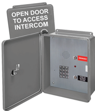
Model Number: 976GIP Dimensions: 11-7/16" H x 13-9/16" W x 5-1/4" D Enclosure: Gray, NEMA 4 Fiberglass, Surface Mount
