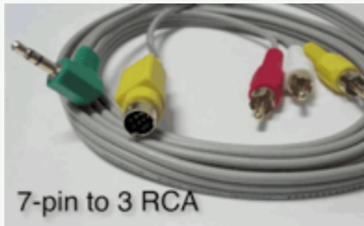
7-Pin S-Video with 3.5mm to 3 RCA
