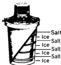
C. When tub is half full, (approx. 2 layers of ice and salt) pour one cup of cold water over the ice and salt mixture. This will help the ice to melt and settle, which will shorten freezing time, and will help keep ice from jamming and causing stops. After tub is filled, pour another cup of cold water over the ice and salt.
