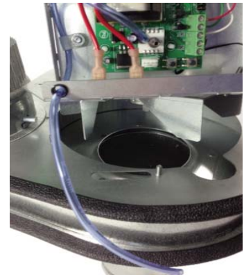
CAREFULLY REMOVE MOTOR / IMPELLER ASSEMBLY.
