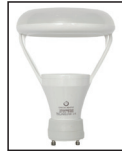
(1) 11 Watt GU24 base LED lamp/2700 Kelvin Warm White/>90CRI/750 lumens/68 LPW/ ENERGY STAR 2.0 certified/25,000 hours rated average life.
