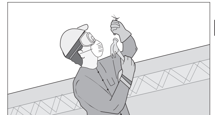
Fig.5. Make an initial hole.
