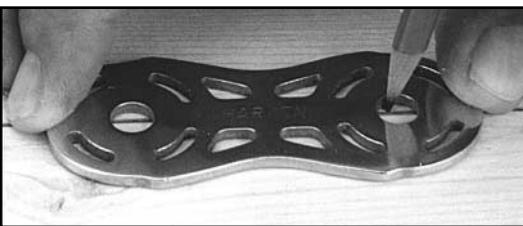
Sandwich two organizer pulleys (E) between two organizer plates (F). Mount in middle of 2" x 6" (50 x 152 mm) board using supplied 1/4" x 2 1/2" (6 mm x 63 mm) lag bolts (G) and washers (H).
