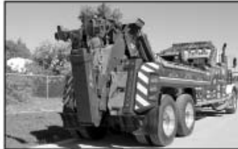
When not in use, the under-reach component is stored in the upright position.
