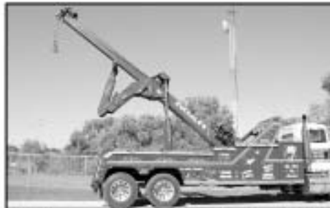
The boom can also be elevated in the extended position.
