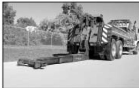
The under-reach can be extended and lowered to ground level when needed.
