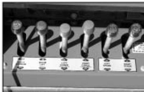
The operator can use truck mounted controls or remote controls to control each function.
