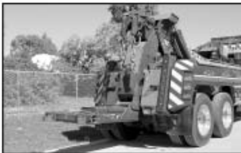
The under-reach can be used to lift heavy vehicles like buses and trucks.
