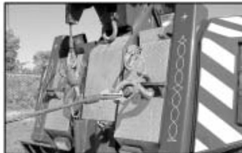
When using the block, rear mounted recovery anchors are used.
