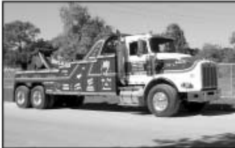
This vehicle is classified as a 50 ton, Class D Recovery Vehicle.
