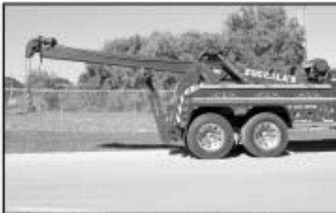
To reach out for an overhead lift, the boom can be extended.
