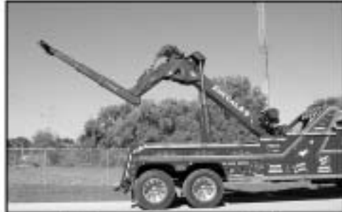
The boom pistons are used to lift.
