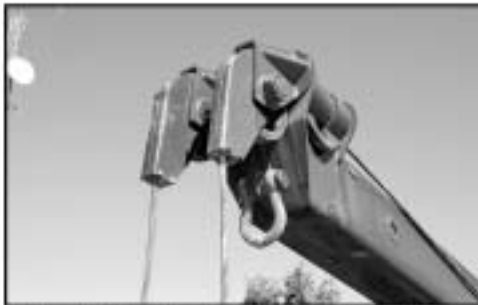
The end of the boom is outfitted with dual boom sheave cable guides.
