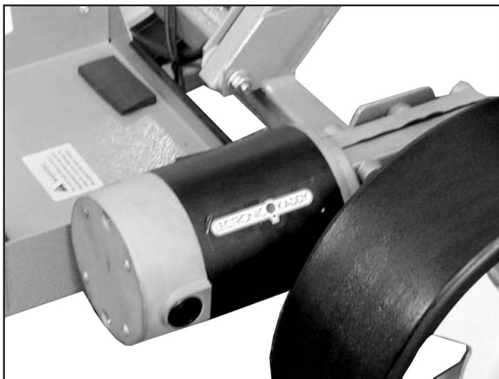
The quality of this motor is obvious when you examine the castings on the motor and gearbox housings. What we especially like is that the motor is designed with replaceable carbon brushes housed in separate brush boxes. This design is similar
