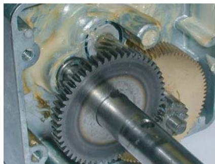
plastic molding. The Dynasteer's gearbox, however, consists of inline steel spur gears and a steel and bronze helical gear primary
