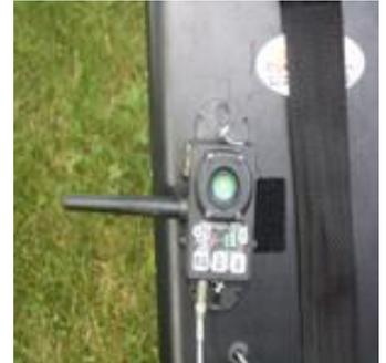
**Note:** When using a dogtra receiver be careful not to let the wire fall inside the machine. If it does you will need to remove the case to retrieve. BE CAREFUL NOT TO STRIP THE SCREW HEADS WHEN REMOVING COVER.
