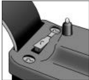
Protection cap not fitted properly. Moisture and debris can enter charging jack.
