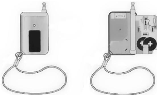
1. Unscrew the small screw on the back of the Remote Control unit.
