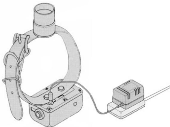
To charge the battery, plug the charger into the battery receptacle on the collar and plug the adapter into any standard 110 Volt household wall outlet. (A 220 Volt European adapter is available from D.T. Systems).
