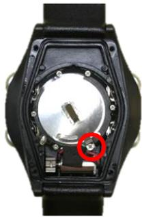
4) Remove the old battery from the watch. Insert a new CR2032 battery with its text facing up.
