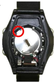
6) Secure the battery bracket with its screw. Make sure the wires are not being pinched.
