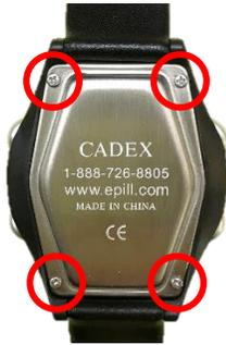
2) Remove the backplate. The sound maker is adhered to its inner face. Leave the O-ring in place.
