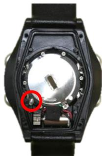
8) Orient the backplate so that 'CADEX' is facing the band's silver buckle. Secure the backplate with its 4 screws.
