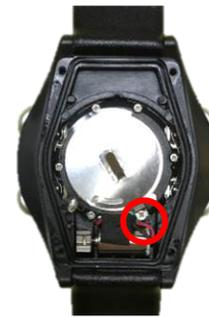
7) Make sure the battery bracket's clear plastic film is not covering the top of the spring.
