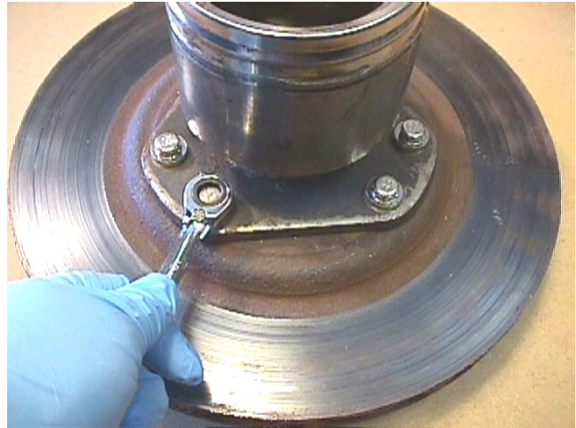
Picture 2 – Install Bolts
